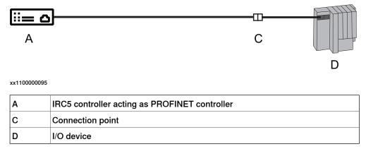
In this alternative there is a direct cable between the PROFINET controller and the I/O device. Enable fast device startup and select 100 MBit (full duplex) on the port. A crossed Ethernet cable needs to be used.
